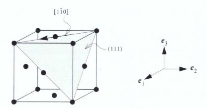
In terms of components with respect to the orthonormal basis  $\{e_i\}$  (i = 1, 2, 3) this  $(111)[1\bar{1}0]$  slip system is characterized by the slip plane normal vector  $\mathbf{m}$  and slip direction  $\mathbf{s}$  given as
